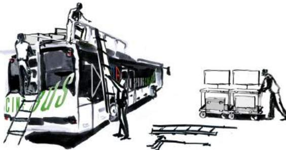
A storage rack on the roof, up to 1000 kg. Possibility of loading log elements (large tripods, jib arm, rails).
