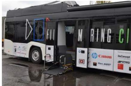
The hydraulic lift facilitates loading weights of up to 500 kg (dolly).
